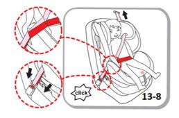
WARNING! MAKE SURE THAT THE VEHICLE BELTS ARE NOT TWISTED AND ARE CORRECTLY FITTED!
