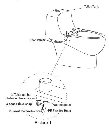
Caution: Take out the U-shape blue snap joint, and then insert the flexible hose, after that, press the snap joint back.
