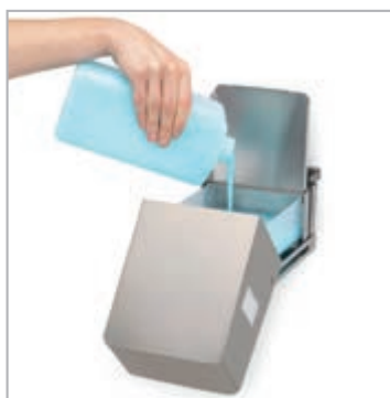
NSU 7 - to be filled from above
